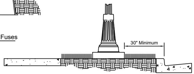
Detail - Pole Spacing From Face of Curb
